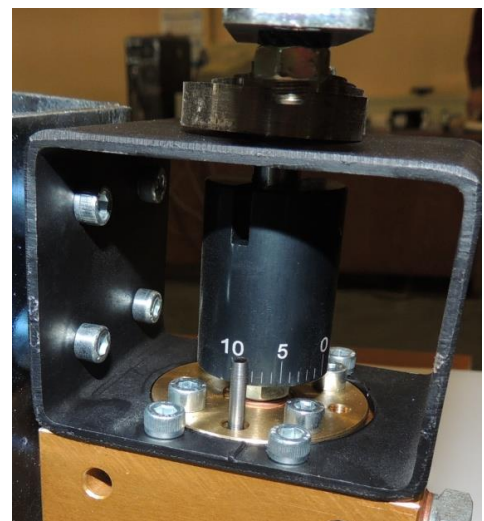
Start position for fuel regulator
